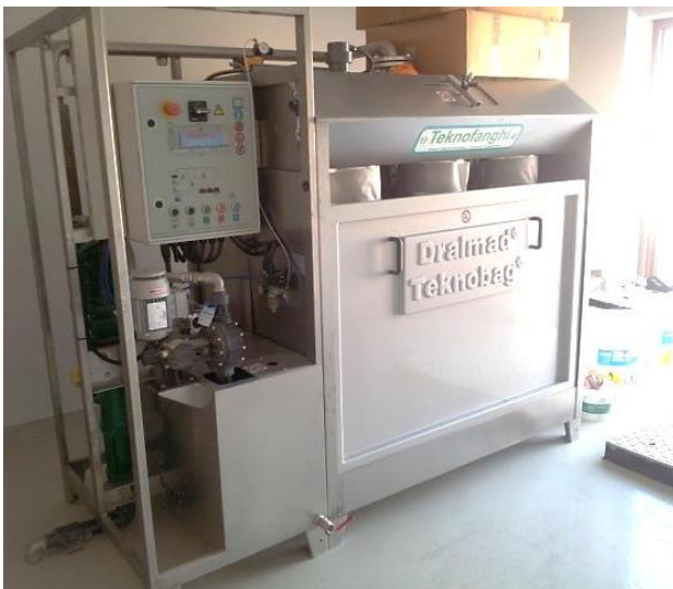
Dry Bag Sludge Dewatering
