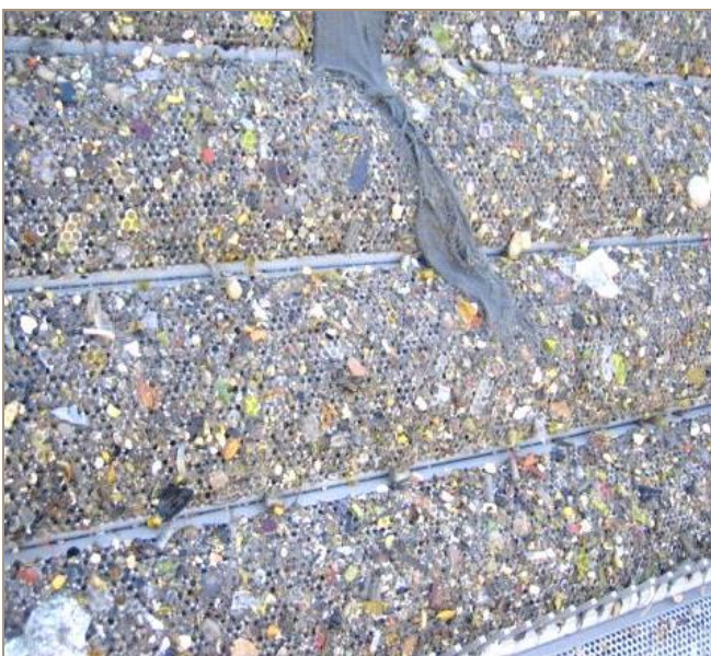
filtered fine particles out of the wastewater
