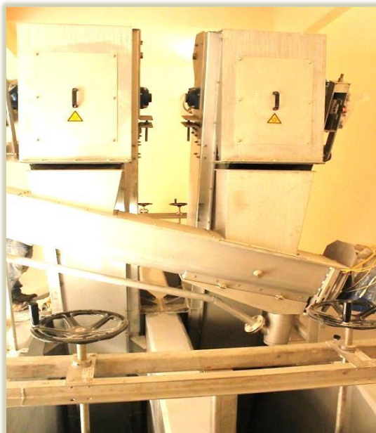
1 x Screening Washing Conveyor
