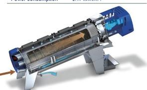
power consumption was less with only 75% than needed with the dewatering centrifuge. This is showing a clear path how to improve the carbon foot print of the plant. Q-PRESS installations can easily achieve a sludge volume reduction in excess of 90% with simple operation and low maintenance at minimum energy consumption. Furthermore, direct dewatering of the thin sludge avoids all additional costs that would incur for the operation of an upstream mechanical thickening system.
