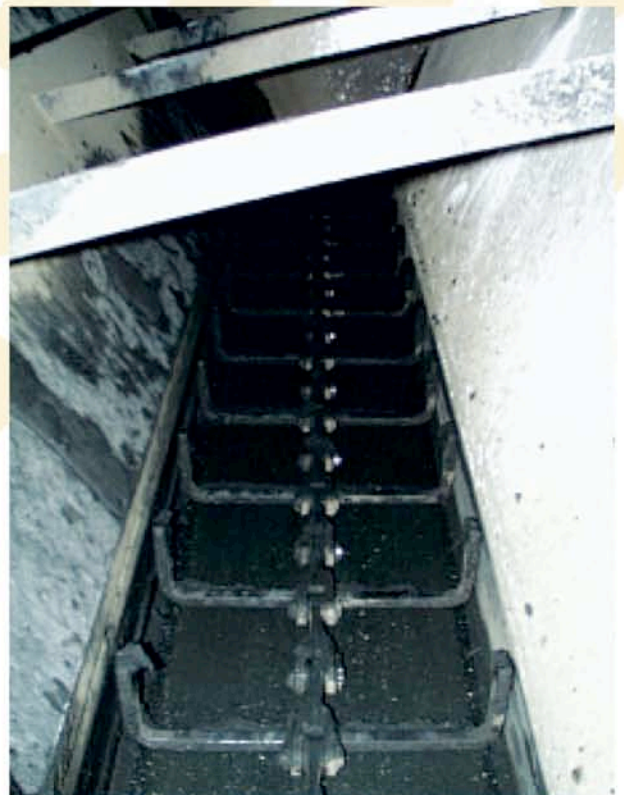
Water Plant Leuna-Daspig Conveyerment and storage of dewatered river sludge.
